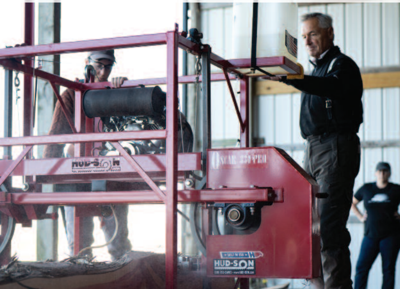
LEFT: At TBC Farm's portable sawmill, Marissa Beinhauer (left) and FFI Woodland Instructor Rick Thomas (right) guide the blade across a cedar log in the Farm & Forest Institute's 1-day "Logs to Lumber" workshop.
